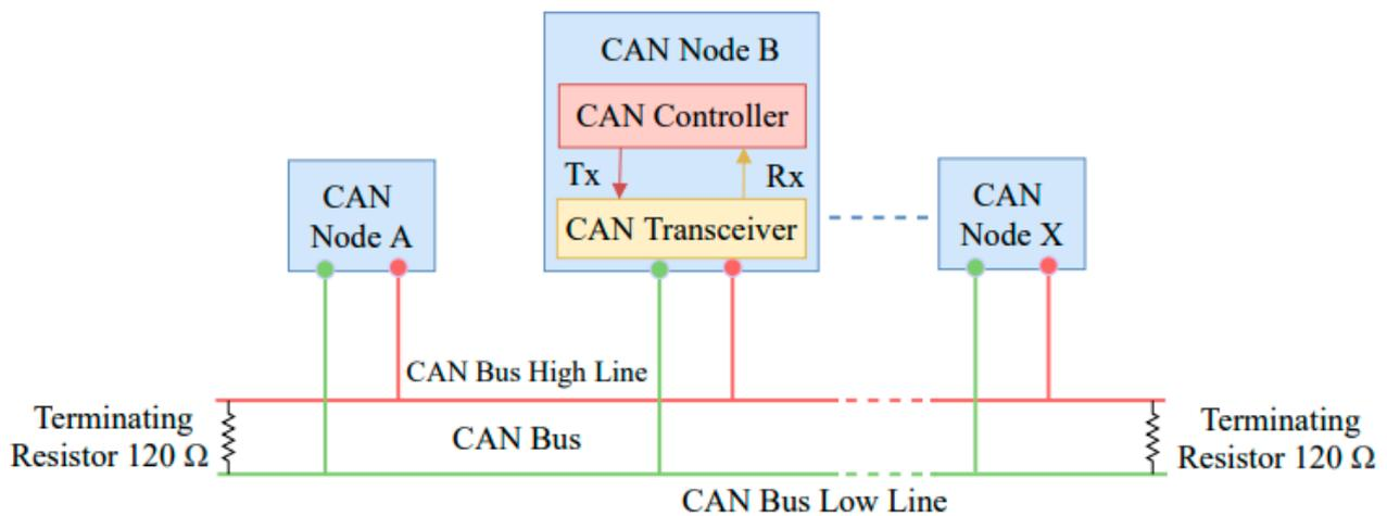
Figure 1. The CAN bus interface.
