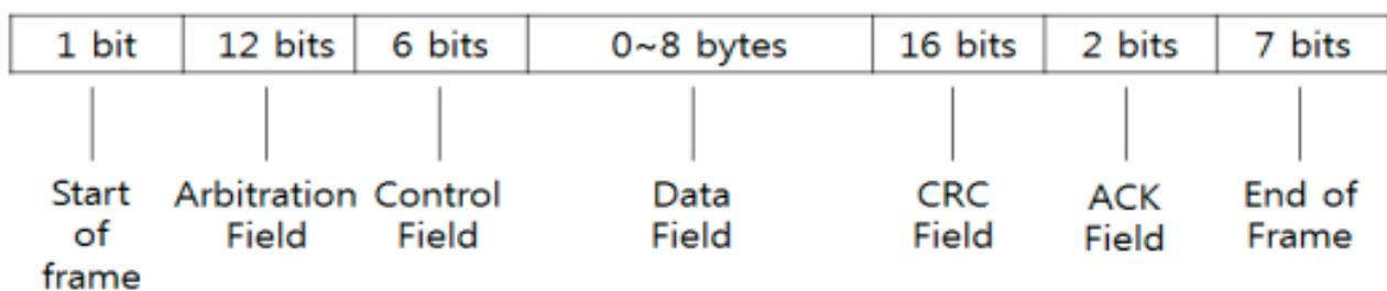
Figure 2. CAN bus data Frame.
