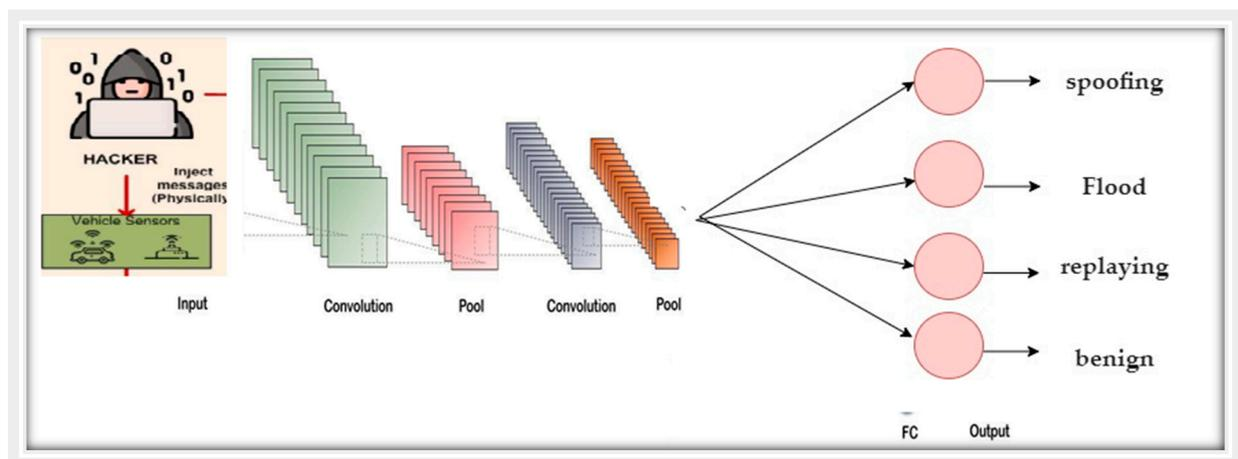
**Figure 6.** The structure of the CNN model.
