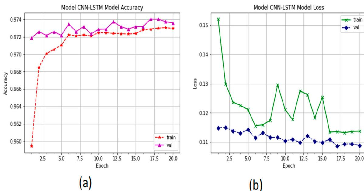
**Figure 13.** The performance of CNN-LSTM: (a) accuracy performance and (b) training and validation loss of the CNN-LSTM model in detecting flood, fuzzing, and normal packets in a CAN bus.
