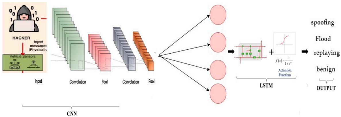
**Figure 7.** The structure of the CNN-LSTM mode.
