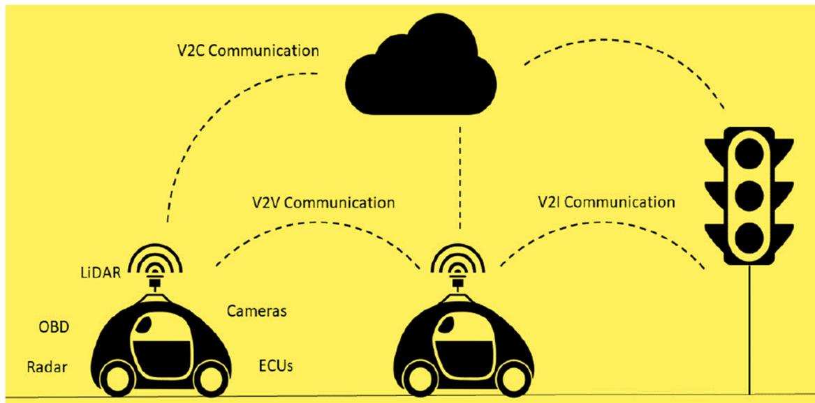
**Figure 3.** Attack points through communication.
