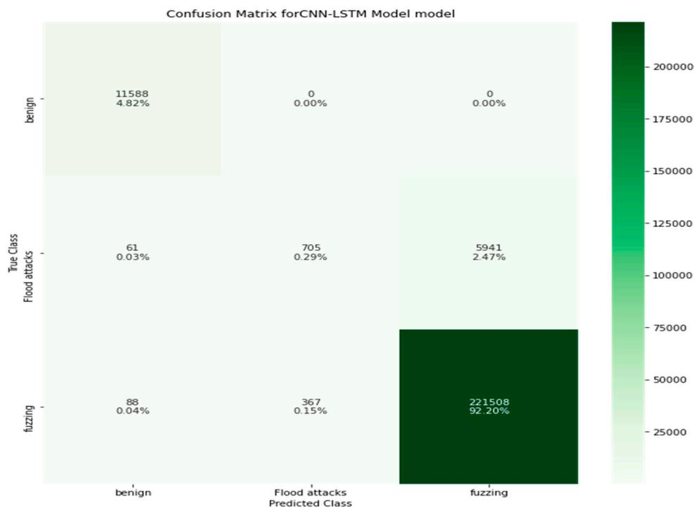
**Figure 12.** The confusion metrics of the CNN-LSTM model in the detection of the flood, fuzzing, and normal packets in a CAN bus network.
