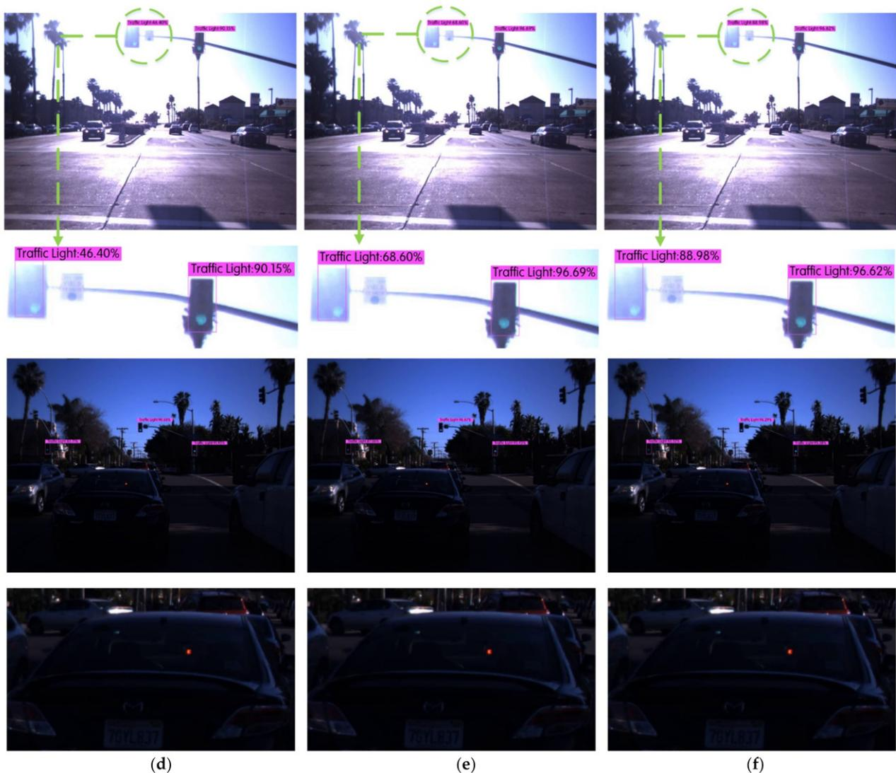
**Figure 9.** Comparison of detection results using multiple algorithms for traffic lights in different scenarios in the LISA data set. (a) Faster R-CNN. (b) YOLOv3. (c) YOLOv4. (d) YOLOv4-v1. (e) YOLOv4-v2. (f) Improved YOLOv4.
