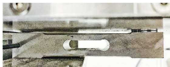
Figure 1. A load cell representation (left) and the load cell used in our device (right).
