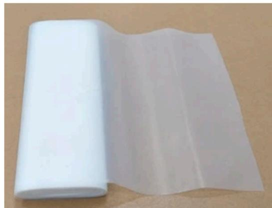
**Figure 9.** Polytetrafluoroethylene (PTFE) films with a thickness of 40 microns.
