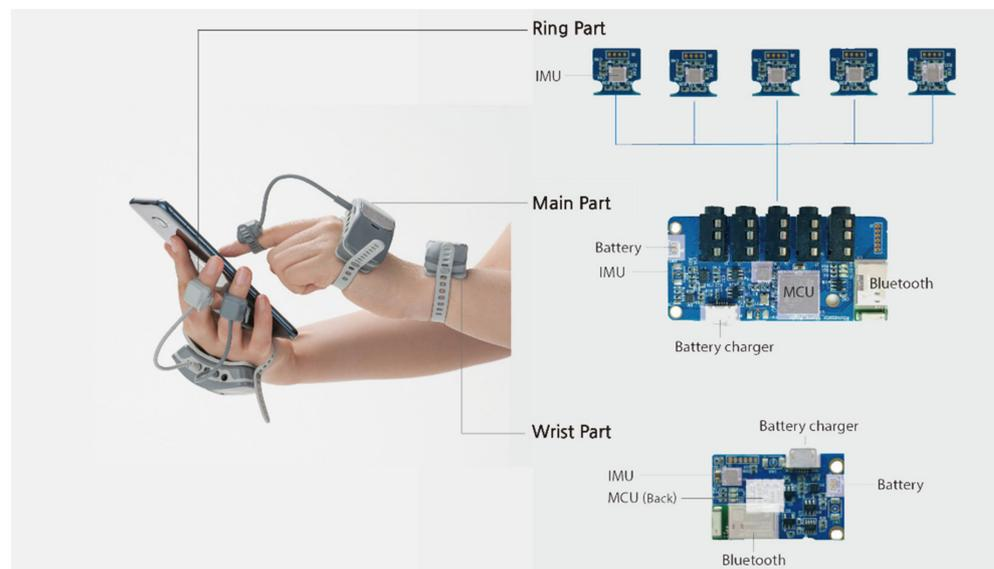
**Figure 1.** Wearable inertial measurement unit (IMU) system for collecting hand movement data during object manipulation.
