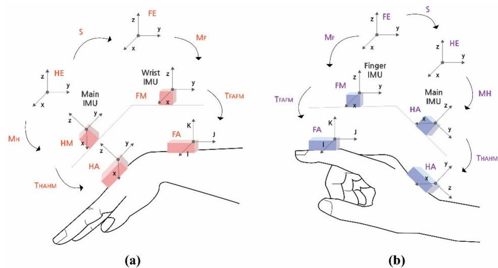
**Figure 2.** A coordinate system related to joint angle estimation: (a) hand to wrist; (b) finger to hand [27].
