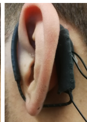
Figure 4. Initial (1st design on the left ) and final (2nd design on the right ) design of the behind-the-ear piece with embedded conductive silicone electrodes.
