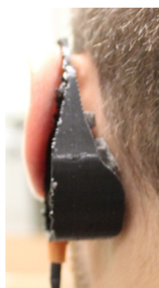
Figure 4. Initial (1st design on the left ) and final (2nd design on the right ) design of the behind-the-ear piece with embedded conductive silicone electrodes.
