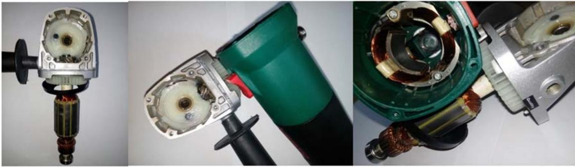
**Figure 6.** Parts of angle grinder (commutator motor, stator, fan, bearing).
