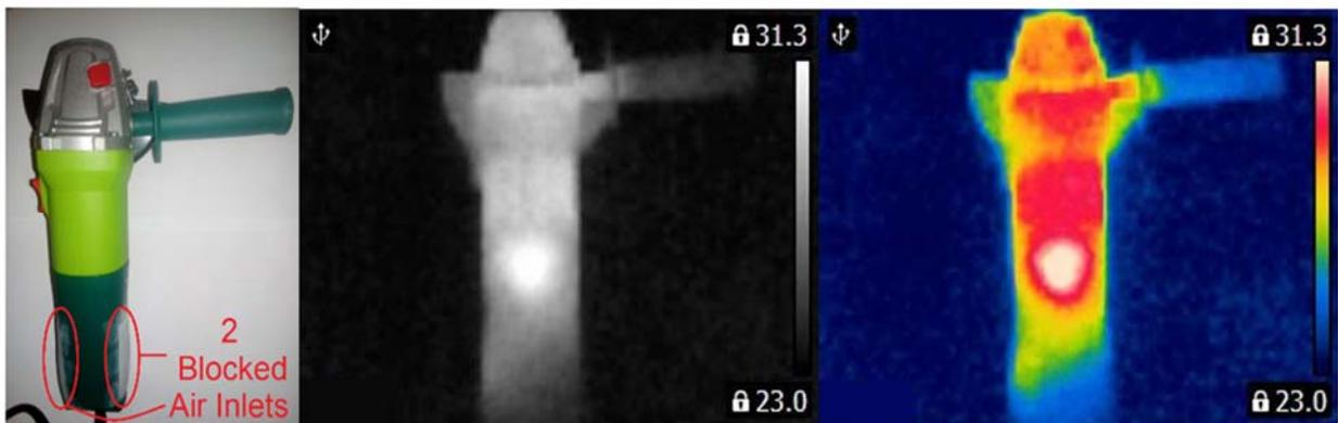
Figure 5. Angle grinder with 2 blocked air inlets.
