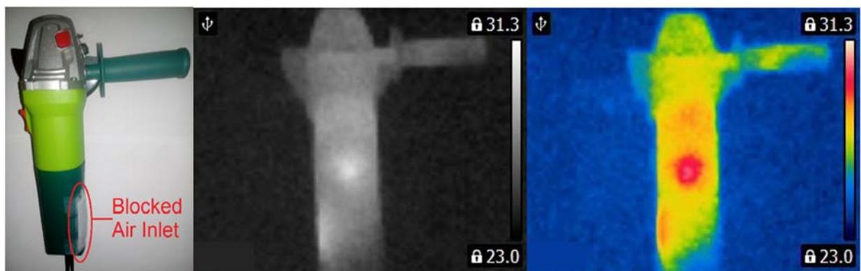
Figure 4. Angle grinder with 1 blocked air inlet.
