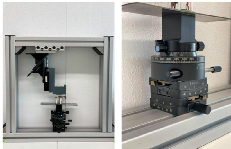
**Figure 4.** Experimental setup with a rotating table, two tilting tables, and slider to adjust the material being tested.
