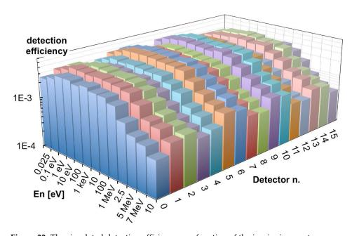
**Figure 22.** The simulated detection efficiency as a function of the impinging neutron energy for the 16 detectors in the  $4 \times 4$  array configuration in the top position.
