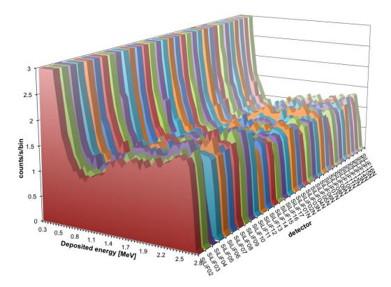
**Figure 10.** The characteristic spectrum shape, measured for all the SiLiF detectors in the front position, is due to the superposition of the triton (2.73 MeV) and alpha (2.05 MeV) contribution smeared down by the effect of the emission from different depths/angles in the <sup>6</sup>LiF converter. The energy bin size is 47 keV.
