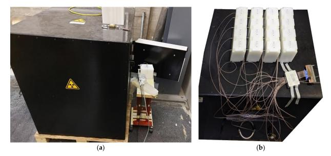
**Figure 6.** (a) The AmBe neutron source box with a SiLiF detector during a measurement in the front position. (b) The  $4 \times 4$  array of SiLiF detectors during the measurement in the *top* position.
