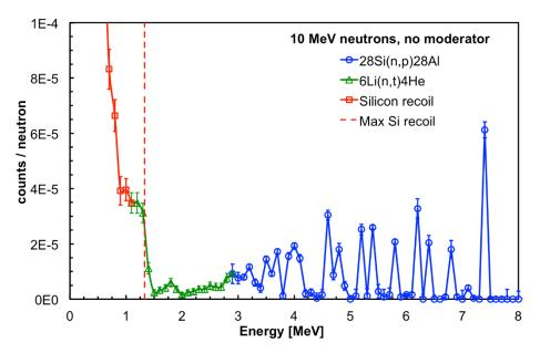
**Figure 13.** GEANT4 simulation of the SiLiF response to 10 MeV neutrons without the moderator surrounding the detector (see text).
