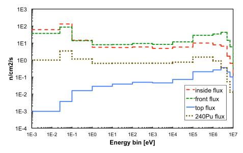
**Figure 9.** Neutron flux simulated in the three measurement positions with Fluka, and with MCNP on the detectors in the radwaste package exercise with <sup>240</sup>Pu (see the Discussion section).
