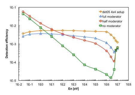
**Figure 5.** Simulated neutron detection efficiency in different moderator configurations (see the text for details).
