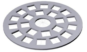
**Figure 2.** Figure **2.** Sketch of the rotating support explicitly constructed for the evaporation of the <sup>6</sup>LiF converters in order to guarantee the uniformity of the deposition.
