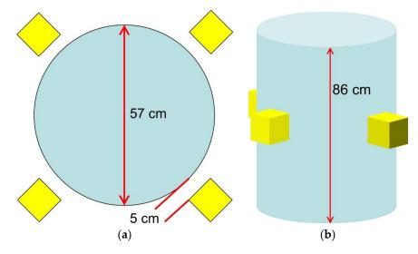
**Figure 24.** Sketch of the simulated radwaste package along with four SiLiF detectors around it. (a) Top view; (b) perspective view.
