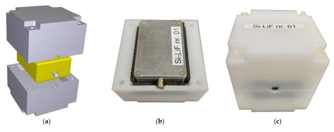
**Figure 4.** (**a**) 3D sketch of the SiLiF detector (in yellow) and its arrangement within the moderator (in grey); (**b**) a SiLiF hosted in a half moderator; (**c**) final assembling of a SiLiF.
