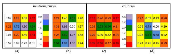
**Figure 23.** (a) Total neutron flux simulated in the *top* position in correspondence of the  $4 \times 4$  SiLiF array; (b) The measured total neutron flux with the  $4 \times 4$  array. (c) The simulated neutron counting rates. (d) The measured neutron counting rates.
