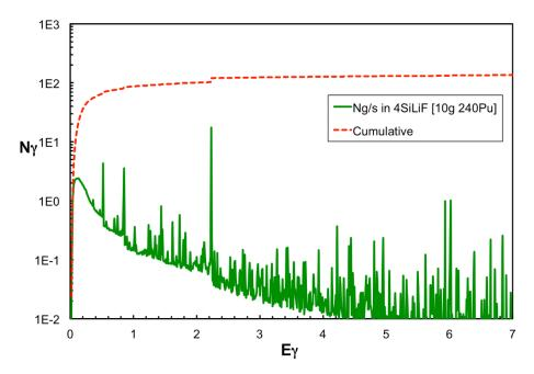
**Figure 25.** The simulated spectrum of the gamma rays impinging on the four SiLiF detectors (green line) and the corresponding cumulative distribution (red dotted line).
