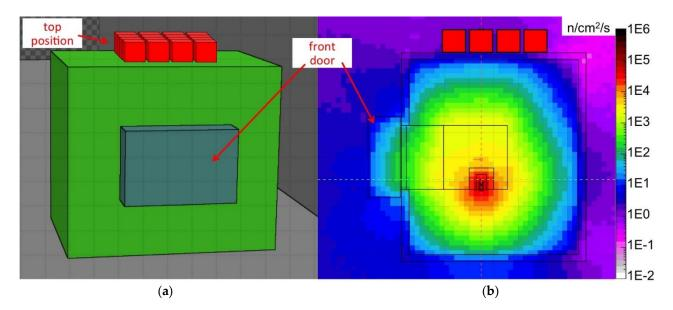
**Figure 8.** (a) Drawing of the 3D side view of the neutron source box, the red box indicates the *top* position; (b) the corresponding neutron flux obtained by means of a simulation with the Fluka code.
