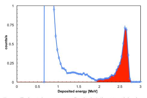
**Figure 15.** The deposited energy spectrum collected in the *inside* position with the reference detector. The colored area starts from the alpha endpoint, and contains 97% of the detected tritons (see text).
