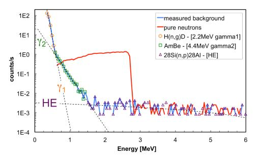
**Figure 11.** The background-subtracted neutron spectrum as compared to the background. Also highlighted are three different contributions to the background (see text).
