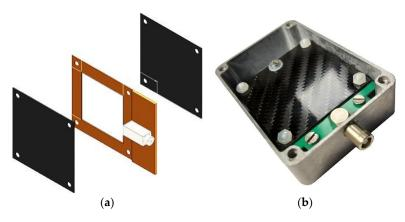
**Figure 1.** (a) The SiLiF detector arrangement as a double sided silicon diode sandwiched between two <sup>6</sup>LiF layers deposited on carbon fiber substrates; (b) a real detector assembled inside its aluminum box.
