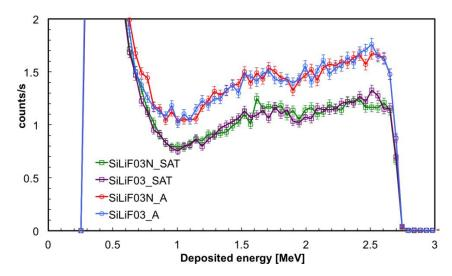
**Figure 18.** Deposited energy spectra obtained with the detectors SiLiF03 and SiLiF03N, belonging to two different silicon batches in the *inside* position. The detectors were coupled with <sup>6</sup>LiF converters deposited onto carbon fiber substrates of the A and SAT types (coming from different manufacturers) which in a second run were swapped.
