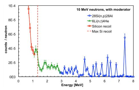
**Figure 12.** GEANT4 simulation of the SiLiF response to 10 MeV neutrons with the moderator surrounding the detector (see text).
