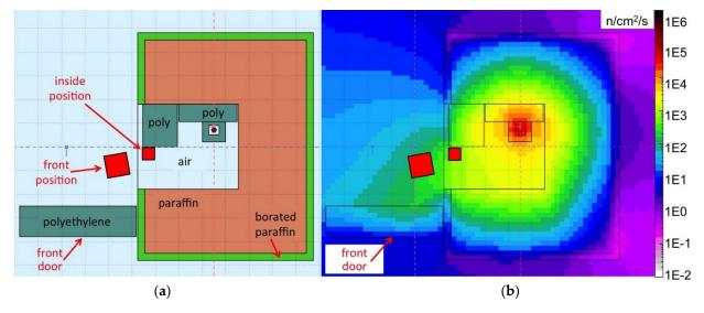
**Figure 7.** (a) Drawing of the top view of the section at 30 cm height of the neutron source box; the source position is indicated by a small dark circle, the red squares indicate the *front* and *inside* positions where the measurements were done; (b) the corresponding neutron flux obtained by means of a simulation with the Fluka code.
