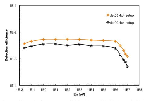
**Figure 21.** Comparison between a corner (det00) and a central (det05) detector simulated efficiency. The overall shapes are similar, the difference being essentially a scale factor enhancement for the central detector due to a geometrical effect of the neighboring moderators.
