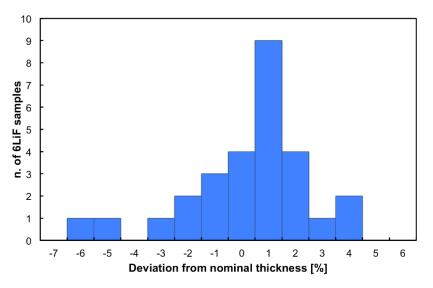
**Figure 3.** Distribution of the deviation of the effective areal density with respect to the nominal value (in percent) for 28 tested samples.
