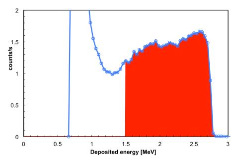
**Figure 16.** The typical deposited energy spectrum collected in the *inside* position with the SiLiF detectors under test. The colored area represents the number of detected neutrons for the chosen 1.5 MeV energy threshold, and was normalized to the impinging flux to provide the detection efficiency for the chosen threshold.
