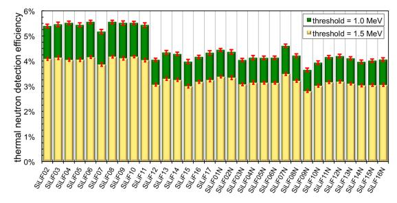
**Figure 17.** The intrinsic detection efficiency measured for the 32 SiLiF detectors in the *inside* configuration, with nominal energy thresholds of 1 and 1.5 MeV.
