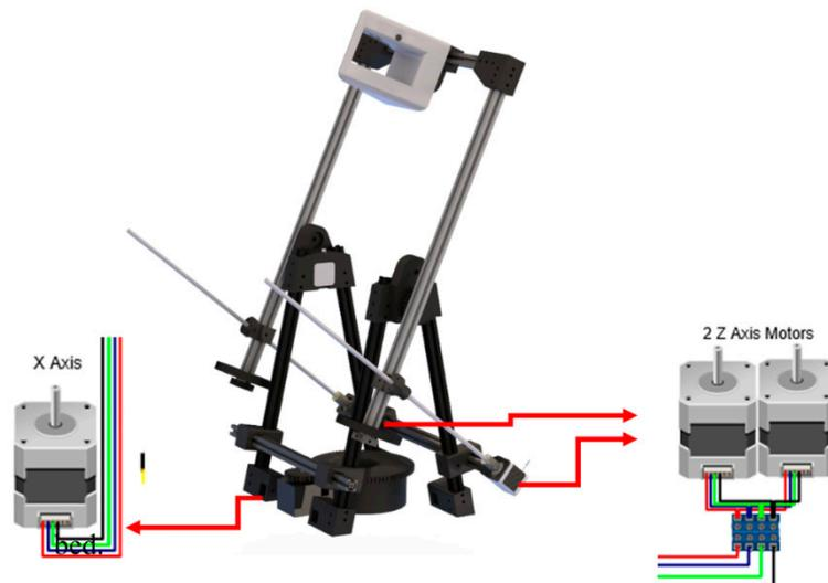
Figure 5. Motors Location. (Source: self-made).
