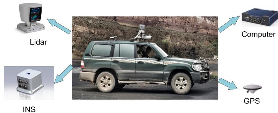
**Figure 23.** Components of the navigation control system.
