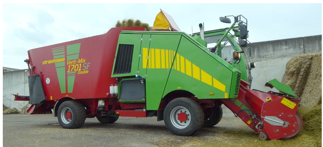
Figure 1. An unmanned feeding mixer is already working with autonomous driving and working functionality. In the developed safety concept, a non-contact sensor system is still missing for the human protection at the autonomous feeding mixer, which may be used both for indoor and outdoor on an agricultural environment.
