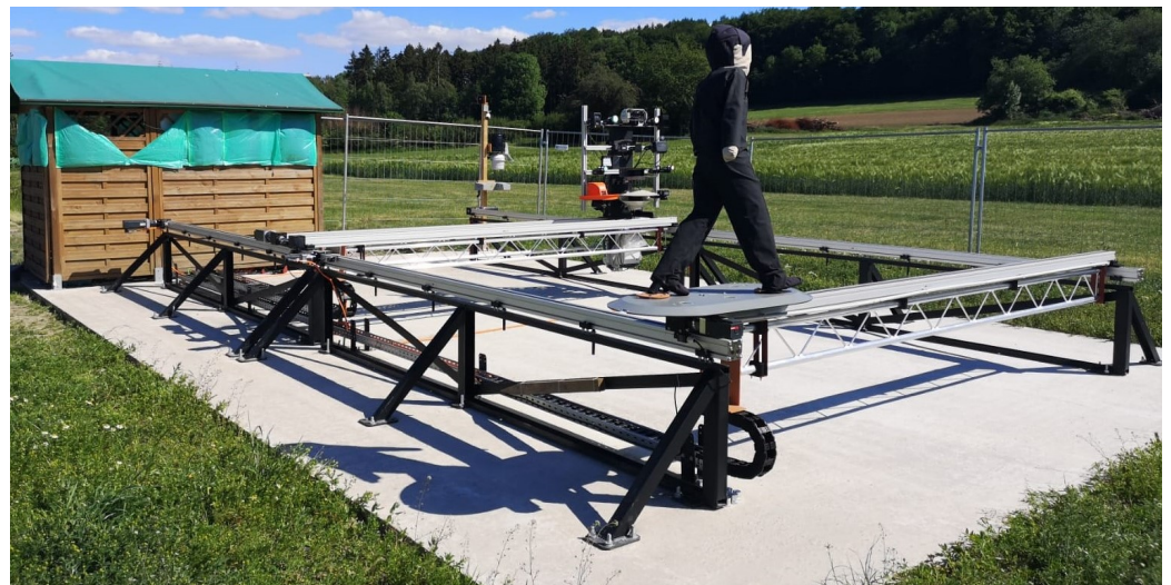
Figure 13. The figure shows the real test stand on an agricultural farm. In the foreground is the test target. Behind it the sensor holder is shown in the figure. Left of the sensor holder the extended weather station with the visibility measuring device and the camera is shown. In the upper left corner of the figure, a hut with the test stand control is shown.
