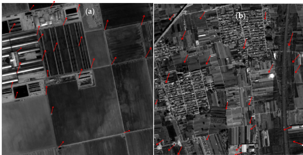
Figure 8. Residuals of the verification results of different orbit data (10× magnification). (a) RMSE of Image 669: 3.25 pixels. (b) RMSE of Image 717: 3.17 pixels.
