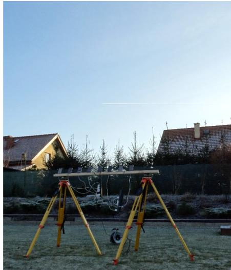
**Figure 1.** Smartphones during GNSS data collection.
