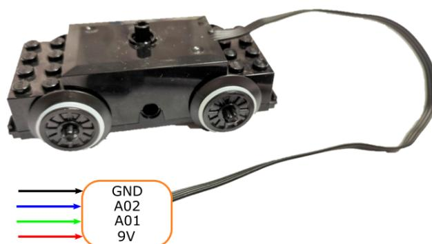
Figure 4. LEGO<sup>®</sup>, Motor wiring diagram.
