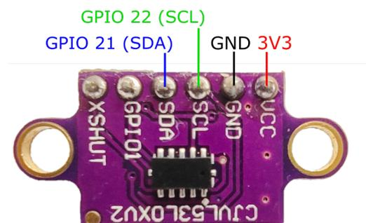
Figure 6. Distance sensor wiring diagram.
