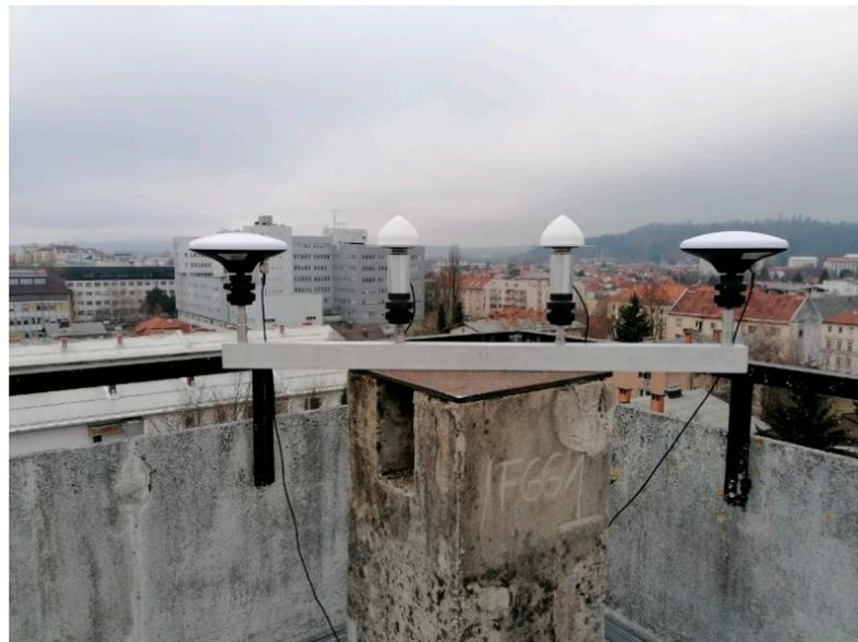
**Figure 3.** Low-cost uncalibrated antennas with the 4-point metal arm.
