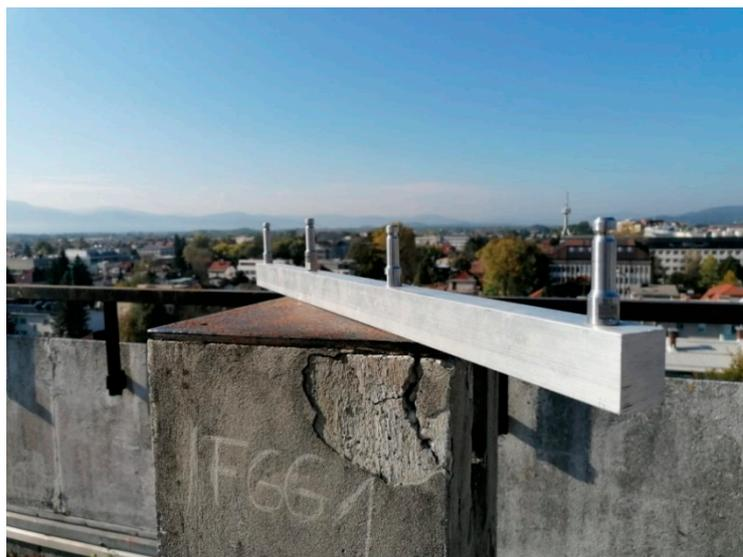
**Figure 2.** The special four-point metal arm used in the short baseline test.
