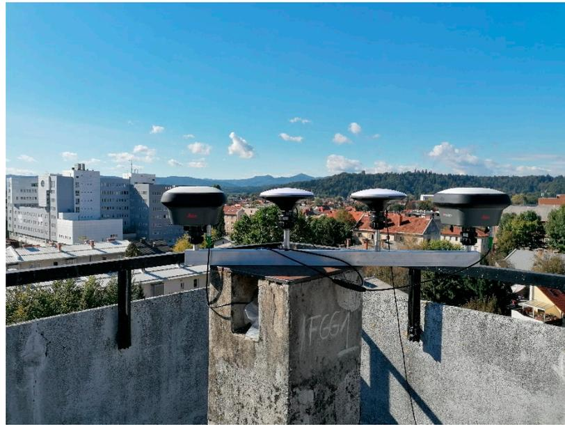
**Figure 4.** Geodetic and low-cost calibrated antennas with the four-point metal arm.
