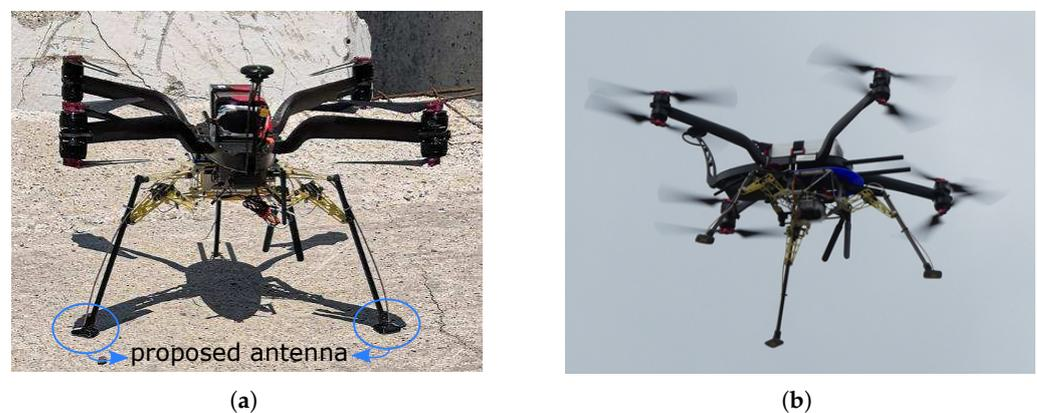
**Figure 1.** Two of the proposed antennas were integrated into an unmanned aerial vehicle (UAV). (a) Landed on the ground; (b) during flight.
