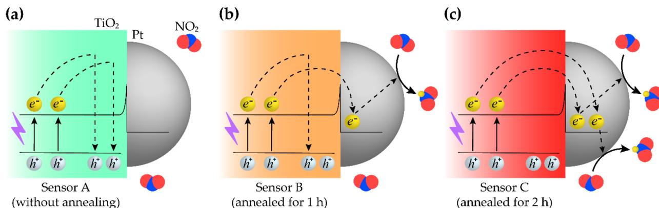
**Figure 7.** Proposed sensing mechanisms are depicted. Photoelectrochemical activities for sensing NO<sub>2</sub> with respect to time of annealing TiO<sub>2</sub> are shown. (a) is the schematic of Sensor A which did not have an annealing process to TiO<sub>2</sub>. (b) and (c) suggest the working mechanisms of Sensor B and Sensor C of which TiO<sub>2</sub> NRs were annealed for 1 h and 2 h, respectively. e<sup>−</sup> and h<sup>+</sup> indicate electron and hole, respectively.
