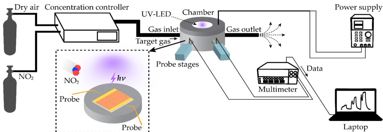
**Figure 2.** An experimental configuration of measuring gas sensing properties is depicted. The concentration controller is a customized system which controls concentrations of the target gas. The inset shows a schematic diagram describing the test chamber. The UV-LED is attached to the top surface. The sample of the gas sensor is laid on the bottom. On the laptop, resistances of the sample obtained by the multimeter are plotted in real-time.
