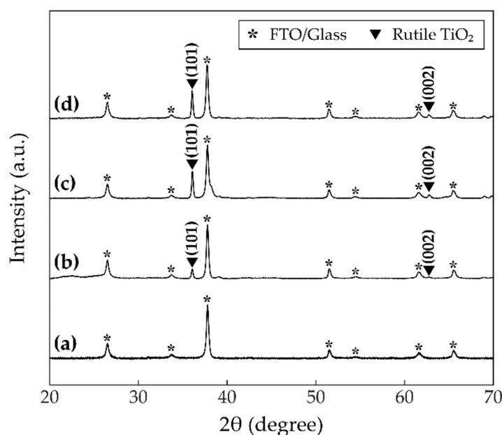
**Figure 4.** X-ray diffraction (XRD) patterns of (a) the FTO-coated glass as the substrate, (b) Sensor A, (c) Sensor B, and (d) Sensor C. The asterisk denotes the peak of the substrate and the triangle marker indicates the peak of the rutile TiO<sub>2</sub>.
