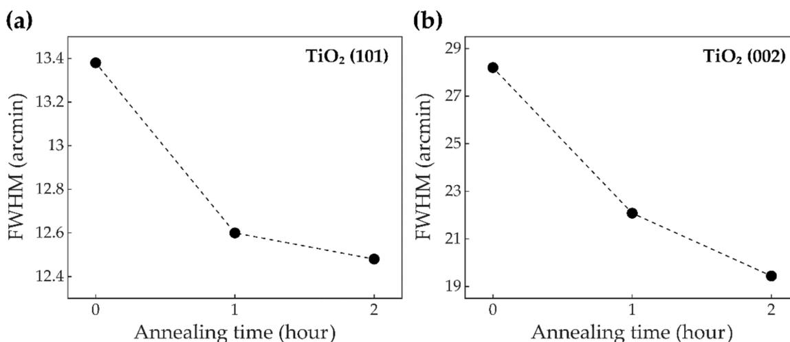
**Figure 5.** The full width at half maximums (FWHMs) of the XRD peaks of the rutile TiO<sub>2</sub> with respect to time of annealing TiO<sub>2</sub> are shown. (a) and (b) are the results at the (101) peaks and (002) peaks in Figure 4, respectively.
