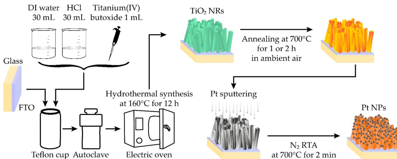
**Figure 1.** A schematic of the fabrication process is illustrated. The hydrothermal method is employed to obtain titanium dioxide (TiO<sub>2</sub>) nanorods (NRs) on the substrate of fluorine-doped tin oxide (FTO)-coated glass. After annealing the TiO<sub>2</sub> NRs, the agglomeration of Pt is utilized by conducting rapid thermal annealing (RTA) to load Pt nanoparticles (NPs) on TiO<sub>2</sub> NRs.
