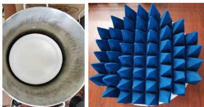
Figure 24. The (left) figure shows the calibration source of aluminum plate, the (right) figure shows the calibration source of absorbing material.
