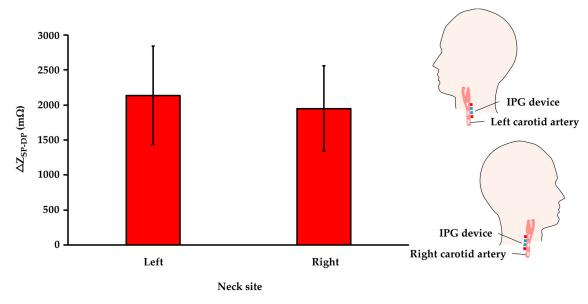
**Figure 9.** The comparison results of IPG measurement resolution between carotid arteries in the left and right sides (n = 6).
