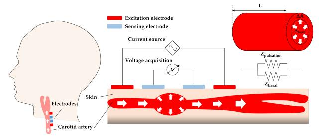
Figure 2. Schematic of IPG-based carotid pulse sensing and equivalent electrical model.
