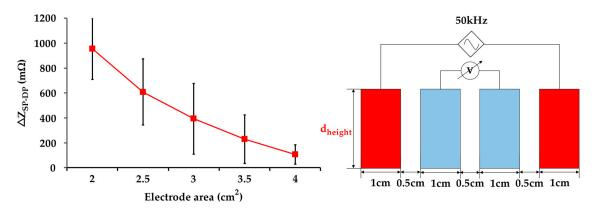
Figure 7. The influence of different electrode cross-sectional areas on IPG resolution measurement (n = 6).
