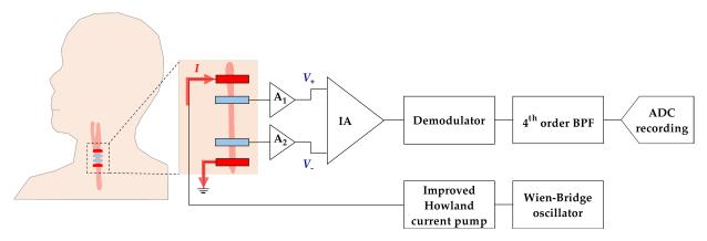
**Figure 3.** IPG system consists of two pairs of electrodes, two pre-amplifiers, instrumentation amplifier, demodulator, 4th order bandpass filter, Wien-Bridge oscillator, and improved Howland current pump.
