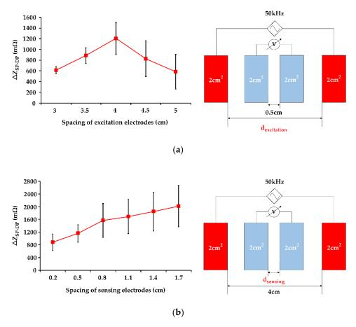
**Figure 8.** The influence of different (a) excitation spacing (from 3 cm to 5 cm) and (b) sensing spacing (from 0.2 cm to 1.7 cm) on IPG resolution measurement (n = 6).
