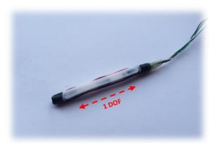
Figure 10. Fiber optic sensor.
