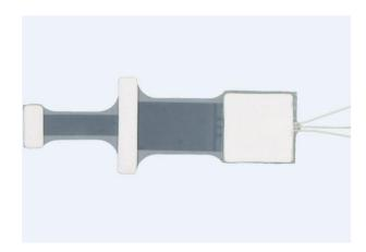
**Figure 13.** StretchSense capacitive sensor [74].
