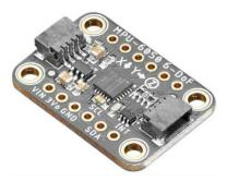
Figure 18. Adafruit MPU-6050 (Breakout Board).
