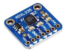
Figure 17. Adafruit ADXL335 (Breakout Board).
