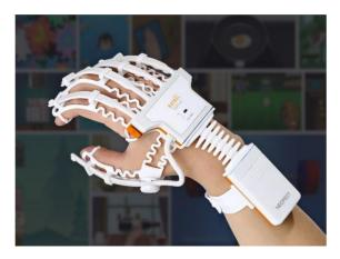
Figure 28. Neofect's Rapael smart glove [93].
