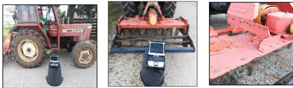
Figure 3. Positioning of the instrument near the machine and accelerometer on the harrow.
