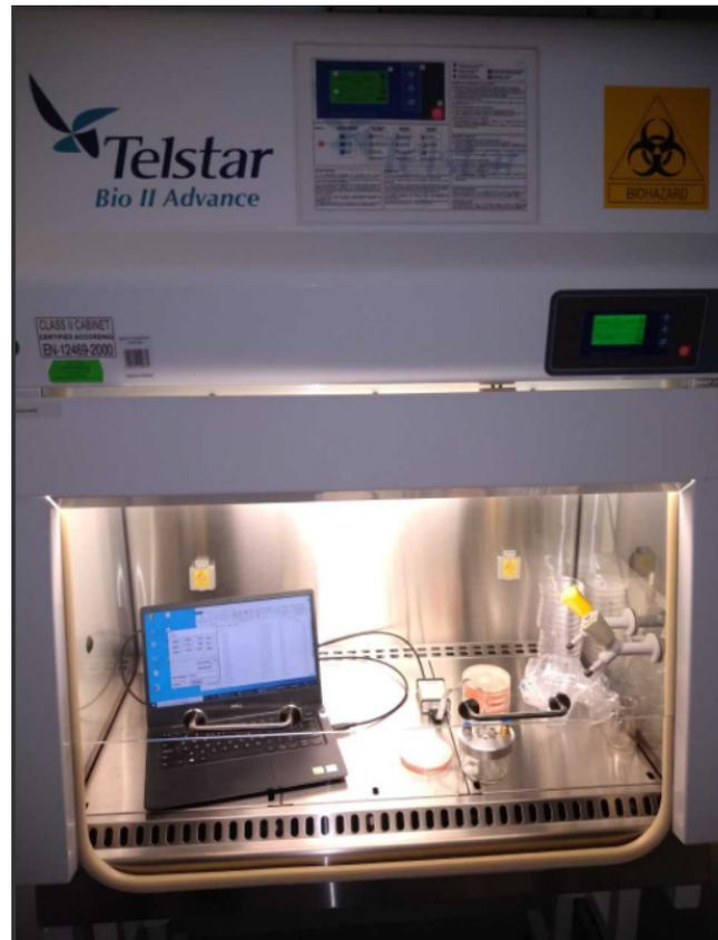
**Figure 2.** Measuring station with the low-cost electronic nose attached to a laptop inside the laminar flow cabinet.
