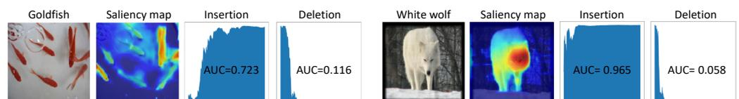
**Figure 5.** Two illustrative examples of calculating insertion and deletion scores in terms area under curve (AUC), each of which consists of an input (leftmost), a saliency map, and insertion and deletion curves.
