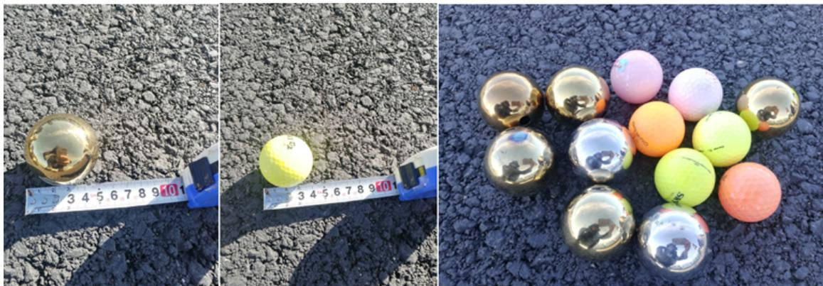
Figure 7. FOD targets used in the experiment.
