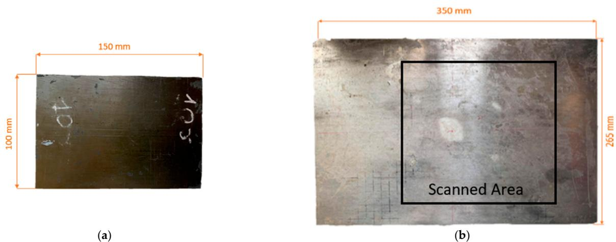
Figure 8. Inspected samples: (a) the carbon-fiber-reinforced (CFRP) polymer  $100 \times 150 \times 4$  mm plate, subjected to a 10 J impact loading in the center, showing barely visible impact damage (BVID); (b)  $350 \times 265 \times 8$  mm aluminium plate with induced stress-corrosion cracks in the centre.
