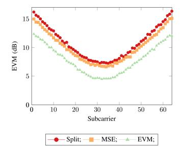
**Figure 5.** Error vector magnitudes across the subcarriers for the three neural network receiver approaches for orthogonal frequency division multiplexing (OFDM).
