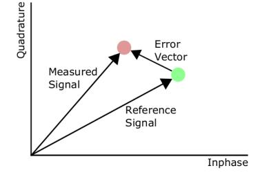
Figure 3. Illustration of error vector magnitude (EVM).
