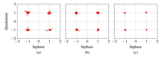
**Figure 4.** Received constellations after neural network processing for (**a**) mean square error (MSE) loss w/Split Complex, (**b**) MSE loss w/Concatenated Complex, (**c**) EVM loss w/Concatenated Complex for spectrally efficient frequency division multiplexing (SEFDM) with  $\alpha = 0.6$ .
