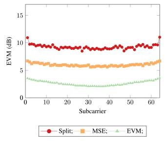
**Figure 7.** Error vector magnitudes across the subcarriers for the 3 neural network receiver approaches for SEFDM with  $\alpha = 0.6$ .
