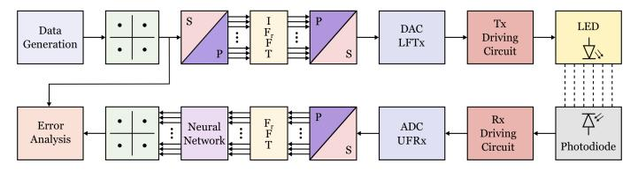
Figure 1. The block diagram of the system used in the experiment.
