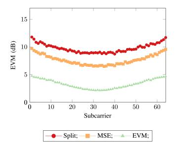
**Figure 6.** Error Vector Magnitudes across the subcarriers for the 3 neural network receiver approaches for SEFDM with  $\alpha = 0.8$ .
