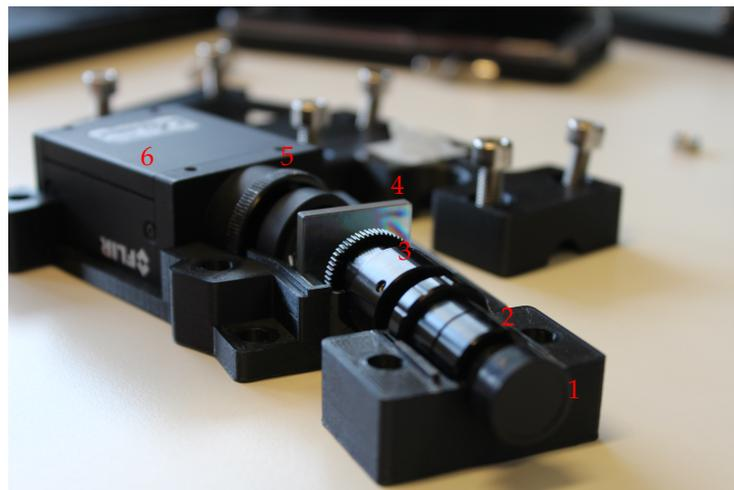
**Figure 1.** Our version of the Sigernes design push-broom imager with the top half removed. Light enters through the front lens (1). Connected to it is the series of S-mounts that contains the slit and the field lens (2), and the S-mount focus tube and the collimator lens (3). Diffraction grating (4) splits the light into its wavelengths. The detector lens (5) is connected to the machine vision camera (6).
