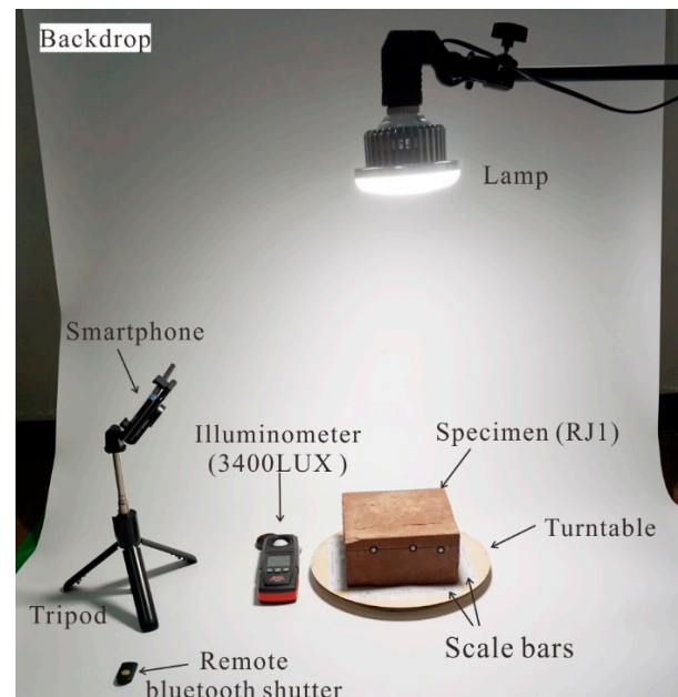
Figure 4. The setup of image acquisition under the FSC mode.
