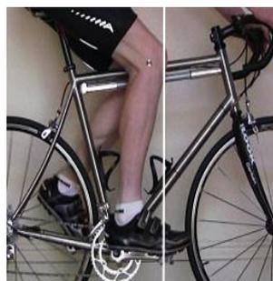
**Figure 1.** Typical KOPS approach to setting saddle height.
