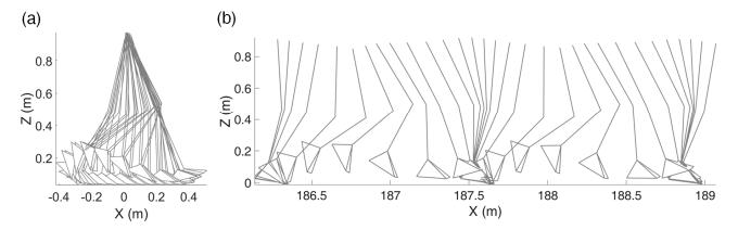
**Figure 1.** Examples of walking trajectory from each system during the same treadmill walking test: (**a**) trajectory from a marker-based optical motion capture (MoCap) system, (**b**) trajectory estimated using inertial measurement unit (IMU) signals.
