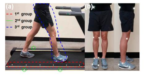
**Figure 2.** (a) Walking test setup with markers attached to a treadmill and a subject; (b) subjectattached markers viewed from the coronal and sagittal planes.
