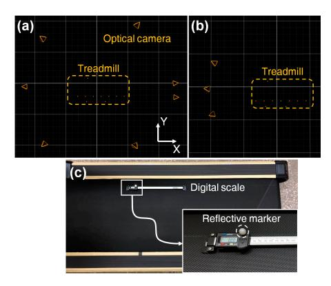
**Figure 4.** Setup for treadmill test without pedestrian walking: (a) camera setting 1, (b) camera setting 2, and (c) setup for evaluation using a digital linear scale.
