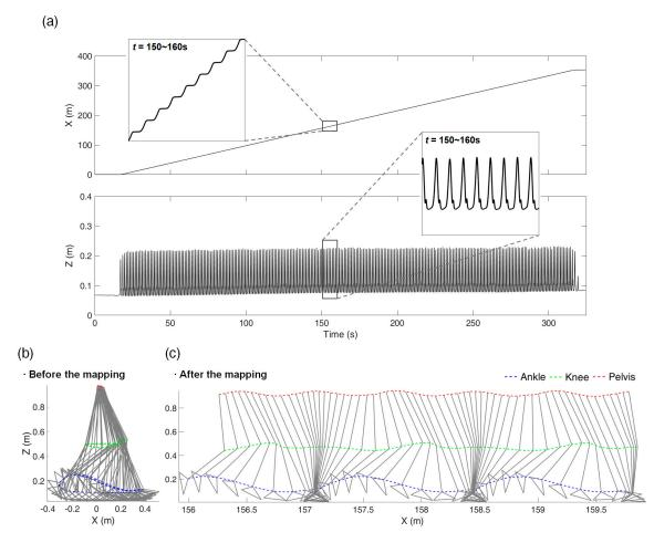
**Figure 5.** Mapping results from Trial 3 of the constant-speed test without inclination: (**a**) shows the *x*- and *z*-axes ankle marker trajectories with respect to time, (**b**,**c**) show marker trajectories on the sagittal plane before and after the mapping, respectively (t = 150-153 s).
