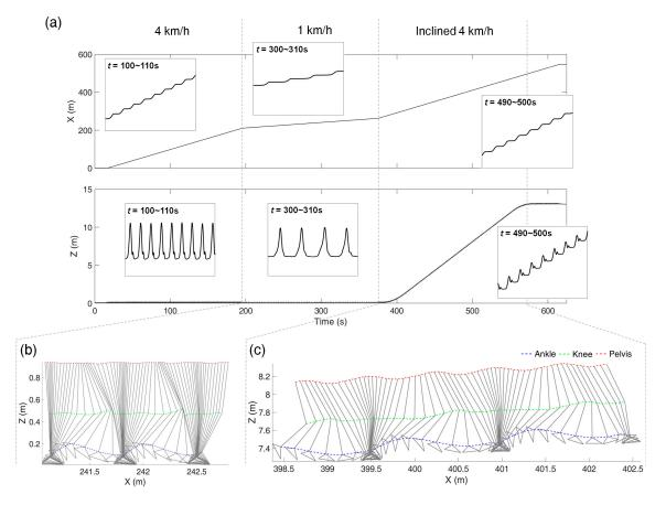
**Figure 6.** Mapping results from Trial 6 of the variable-speed tests with various inclinations: (**a**) shows the *x*- and *z*-axes ankle marker trajectories with respect to time, (**b**,**c**) show marker trajectories on the sagittal plane after the mapping, during 1 km/h walking without inclination (t = 300-306 s) and during 4 km/h with the inclination of 4° (t = 490-493 s), respectively.
