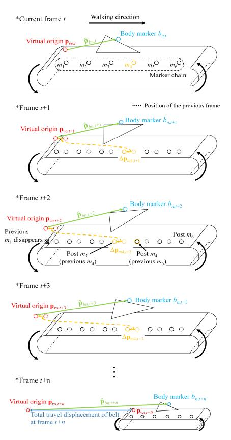
Figure 3. Mapping procedure over the time frame.
