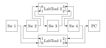
Figure 15. Topology used to measure the end-to-end delay and the jitter in the presence of faults.
