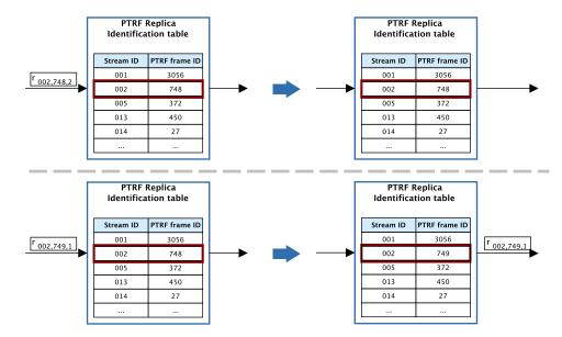
**Figure 11.** This figure shows the operation of the PTRF Replica Identification table. Specifically, on the top of the Figure, we see how the table processes a replica of a message edition that has previously been received. On the bottom, we see how the table processes a replica of a message edition that is received for the first time.
