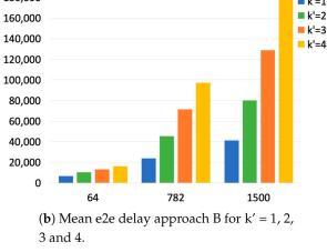
**Figure 16.** Mean value for the maximum end-to-end delay for approaches A and B with k = k' = 1, 2, 3 and 4. The X axis represent the frame length in bytes, while the Y axis represent the end-to-end delay in nanoseconds.
