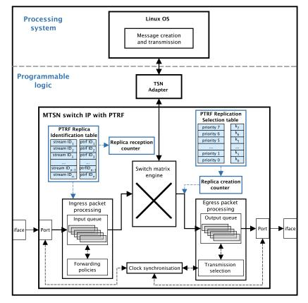
**Figure 12.** Basic architecture of the MPSoC that implements the PTRF mechanism. The PTRF components are highlighted in blue. Solid lines represent the path which frames follow whereas dashed lines represent management or configuration interactions.
