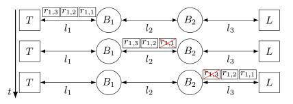
**Figure 6.** Behaviour of the approach B of the PTRF mechanism in the presence of temporary faults in the links.
