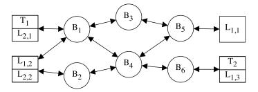
**Figure 3.** An example of a TSN-based network architecture with four end-systems and six bridges in a mesh topology. End-systems are represented with squares, bridges with circles and links with arrows. The T means that the end-system is a talker, while the L means it is a listener.
