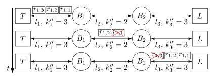
**Figure 7.** Behaviour of the approach C of the PTRF mechanism in the presence of temporary faults in the links.
