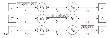
**Figure 5.** Behaviour of the approach A of the PTRF mechanism in the presence of temporary faults in the links.
