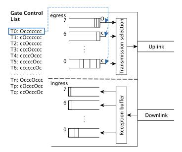
**Figure 2.** Internal structure of a port with Time-Aware Shaper. Each egress queue of the port has a gate that can be configured as open "O", to allow frames to be transmitted, or closed "c", to prevent frames from being transmitted. On the left-hand side of the figure we can see an example of gate control list.
