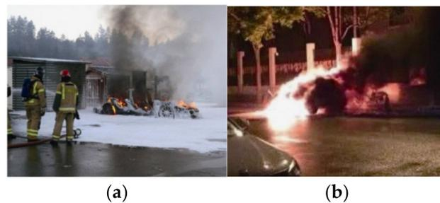
**Figure 1.** Lithium ion battery failure accident of electric vehicle [1]. (a) Battery catches fire when charging; (b) Self-ignition of the battery.
