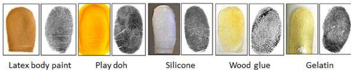
**Figure 1.** Different examples of spooft fingerprints fabricated using different materials. The photograph of the fabricated fingerprint is on the left, and the captured fingerprint image using Crossmatch sensor is on the right [4].
