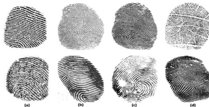
**Figure 5.** Sample images of LivDet2015 dataset. Live samples are in the top row and fake samples are in the bottom row. Samples are from Digital Persona (a), Green Bit (b), Biometrika (c), and CrossMatch (d) sensors.
