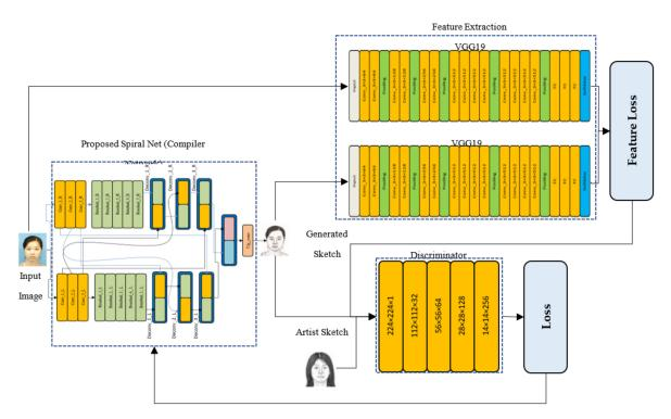
Figure 1. Schematic diagram of the proposed method.
