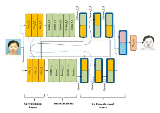
Figure 2. Architecture of Spiral-Net as a sketch compilation network.
