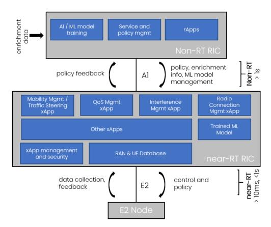
Figure 2. RAN Intelligent Controller: non-RT RIC and near-RT RIC.
