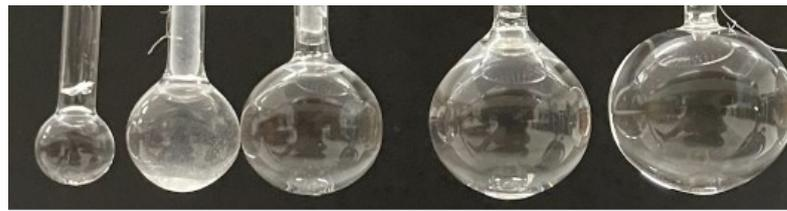
**Figure 1.** The glass tumour bulbs (filled with saline solution) used as tumour surrogates in the breast phantoms.
