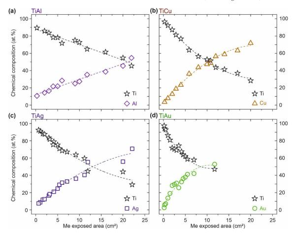
**Figure 3.** Evolution of the atomic composition (at.%) of the four Ti–Me intermetallic systems obtained by RBS spectra analysis: (a) Ti–Al, (b) Ti–Cu, (c) Ti–Ag, and (d) Ti–Au. The connecting dashed lines represent the composition evolution trend of each system.
