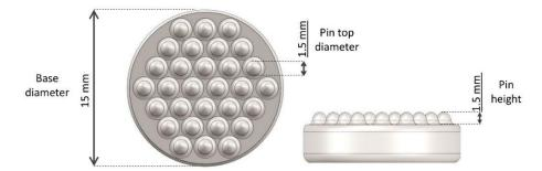
**Figure 1.** Top and side-view of the multiwave PU substrate containing 30 wave pins in a honeycomb configuration. The relatively short waves provide an improved feeling of comfort and ensure proper interfacial electrode–skin contact [15,37].
