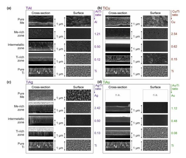
**Figure 5.** Morphology evolution of the Ti–Me films attending to the different structural zones identified: (**a**) Ti–Al system, (**b**) Ti-Cu system, (**c**) Ti-Ag system, and (**d**) Ti–Au system. The morphology of the pure Ti and Me metallic thin films are included to be used as reference.
