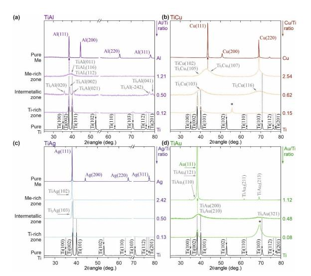
**Figure 4.** X-ray diffraction patterns of the Ti–Me representative films attending to the Me/Ti ratio for every system prepared: (a) Ti–Al system, (b) Ti–Cu system, (c) Ti–Ag system, and (d) Ti–Au system. For Ti–Me systems prepared with Al (a) and Ag (d), a break in the scale of the diffraction angle (*x*-axis) was introduced, to highlight the main crystallographic orientation growths of both systems.
