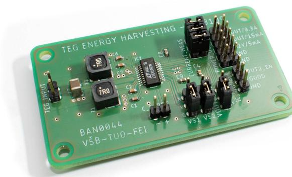
**Figure 7.** Experimental printed circuit board equipped by LTC3109 DC/DC converter.
