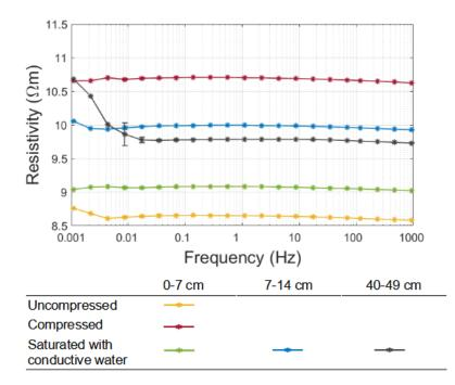
**Figure 9.** Frequency-dependent resistivity of the sediment samples of core Nah-16 I. Samples from 0–7 cm of the core were packed using different procedures (uncompressed, compressed, and saturated with conductive water). Samples from different sections of the core (0–7 cm, 7–14 cm, and 40–49 cm) were packed using the same procedure (saturated with water).
