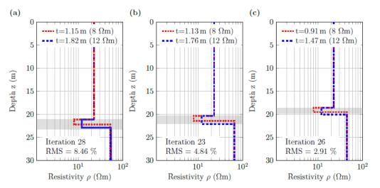
**Figure 15.** Layered resistivity models for ERT data measured at the intersections between ERT line Nah13 and SBP profiles (**a**) L3 NS, (**b**) L4 SN, and (**c**) L5 NS of section A (Figure 1b). The two inverted models correspond to two fixed values of the sediment resistivity (8 and 12  $\Omega$ m); RMS errors indicated in the respective panels are the same for both models. The grey shadings indicate the sediment layer thicknesses derived from collocated SBP profiles.
