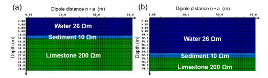
**Figure 10.** Resistivity models used for the modeling study: (**a**) Model with a 1.5 m sediment layer at 10.5 m water depth. (**b**) Model with a 2.5 m sediment layer at 21.0 m water depth.
