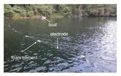
**Figure 4.** Picture of the water-borne electrical-resistivity tomography (ERT) measuring system. The marine resistivity cable with 13 stainless-steel electrodes in the foreground was kept afloat by foam elements attached to the marine cable. The boat with the measuring device in the background also carried the integrated GNSS and echo-sounder device.
