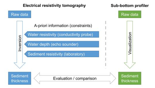
**Figure 2.** Flowchart describing the general approach of this study. The measured ERT data were inverted by using water depth, water resistivity, and sediment resistivity as constraints. The sediment thickness resulting from the inversion was then compared to the sediment thickness obtained from the SBP profiles.
