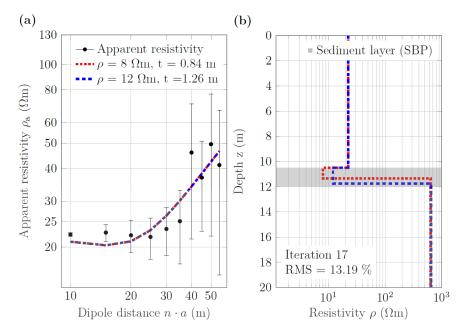
**Figure 16.** One-dimensional inversion of measured ERT data corresponding to the ten current dipoles of section C along ERT line Nah6. (a) Observed (black dots) and calculated apparent resistivity sounding curves. (b) Layered resistivity models for two different values of the fixed sediment resistivity; RMS errors were the same for both models. The grey shading indicates the sediment layer thickness derived from the collocated SBP line L4 SN.
