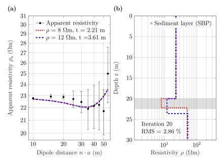
**Figure 13.** One-dimensional inversion of measured ERT data corresponding to the ten current dipoles of section B along ERT line Nah9. (a) Observed (black dots) and calculated apparent-resistivity sounding curves. (b) Layered resistivity models for two different values of the fixed sediment resistivity; RMS errors were the same for both models. The grey shading indicates the sediment-layer thickness derived from the collocated SBP line.
