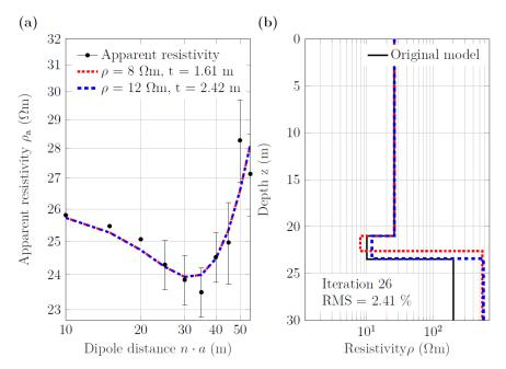
**Figure 12.** One-dimensional inversion of the synthetic data obtained for the sediment layer at 21.0 m depth including synthetic noise. (a) Observed (black dots) and calculated apparent-resistivity sounding curves. (b) Layered resistivity models for two different values of the fixed sediment resistivity; RMS errors were the same for both models. The black solid line represents the original model (sediment layer:  $10.0 \Omega m$ , 2.5 m).
