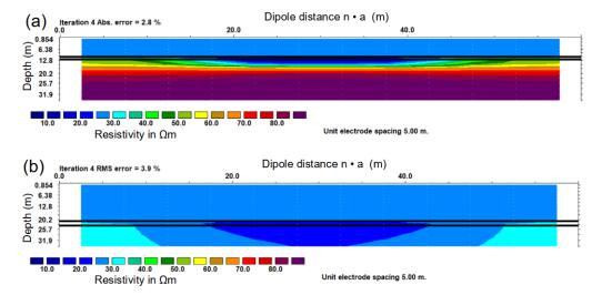
**Figure 11.** Inversion of synthetic data for (**a**) a sediment layer of 1.5 m and 10.5 m water depth and (**b**) 2.5 m sediment layer and 21.0 m water depth. The black horizontal lines mark the upper and lower limits of the sediment layer of the original resistivity model.
