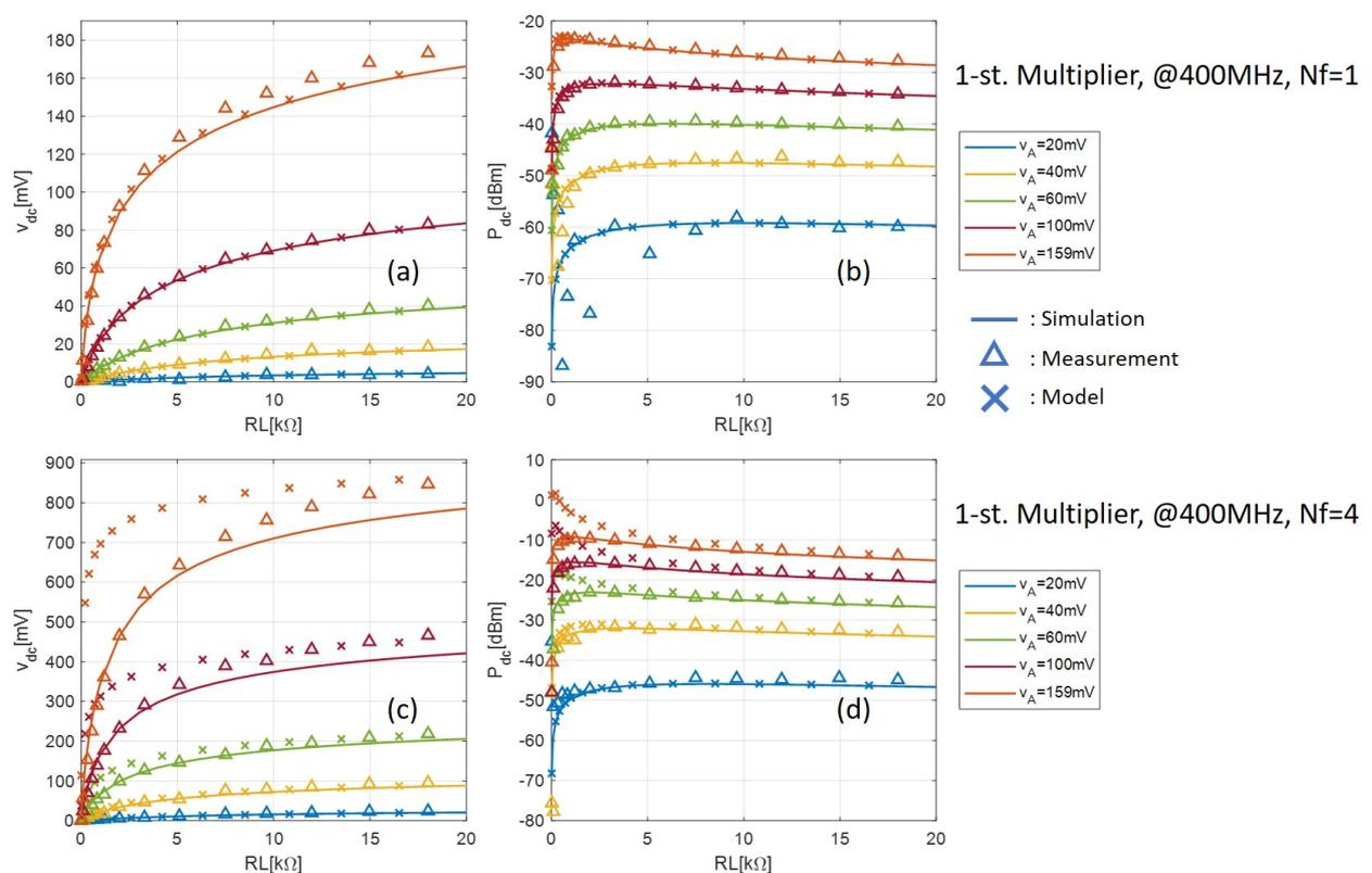
Figure 8. Comparison between measurement, simulation, and analytical model of the one-stage multiplier. Output DC voltage with (a)  $N_f = 1$  and (c)  $N_f = 4$ ; output DC power with (b)  $N_f = 1$  and (d)  $N_f = 4$ .
