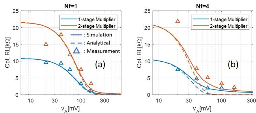
**Figure 10.** Optimal loads calculated by simulation, numerical solution of the analytical model, and measurement with (a)  $N_f = 1$  and (b)  $N_f = 4$ . Note that the measured results with the lowest input tone amplitude  $v_A$  tend to be outliers since the rectifier's output voltage is close to the noise floor of the oscilloscope.
