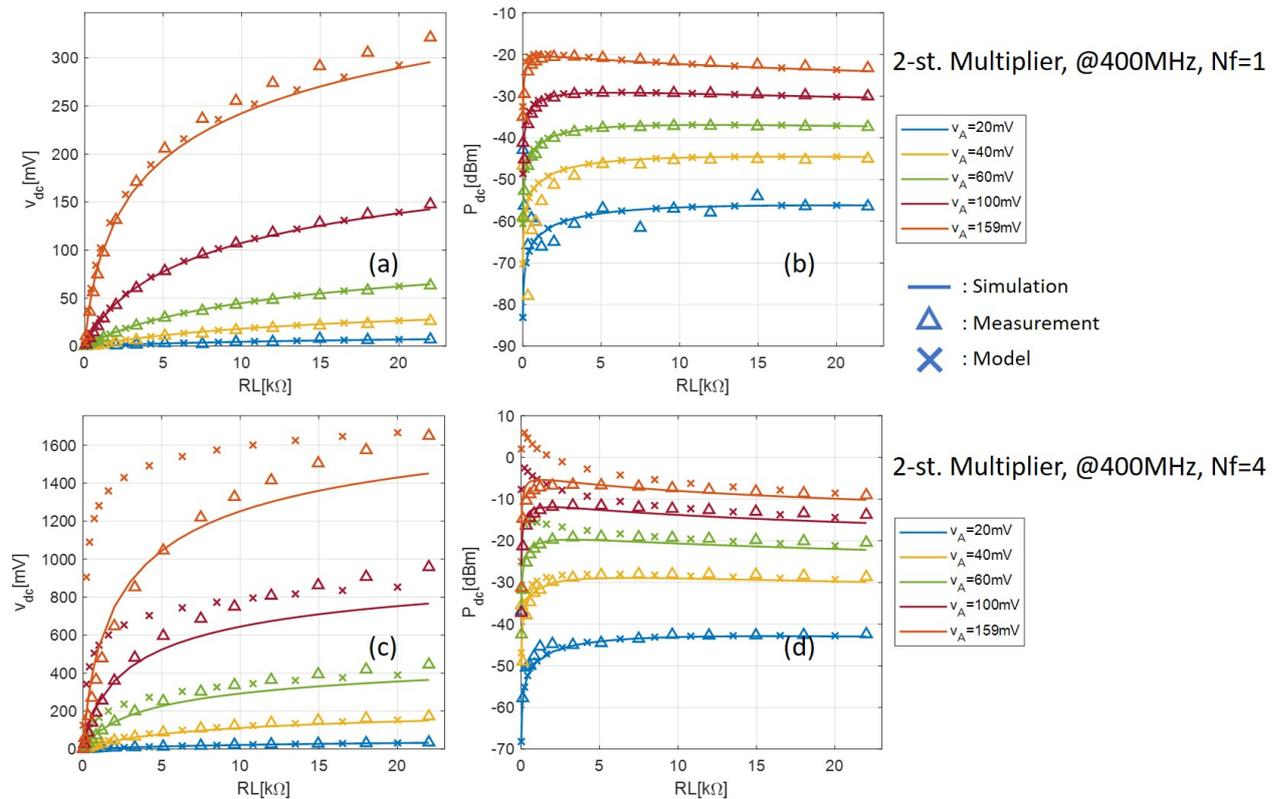
**Figure 9.** Comparison between measurement, simulation, and analytical model of the two-stage multiplier. Output DC voltage with (a)  $N_f = 1$  and (c)  $N_f = 4$ ; output DC power with (b)  $N_f = 1$  and (d)  $N_f = 4$ .
