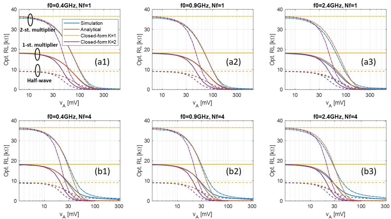
**Figure 4.** Optimal load calculated by transient simulation (blue), numerical solution of the analytical model (red), and closed-form solutions (yellow and purple) when (a)  $N_f = 1$ , and (b)  $N_f = 4$  with  $\Delta_f = 1$  MHz, simulated with half-wave, 1-, and 2-stages voltage-multipliers using Avago HSMS285x. The results under different frequency bands (a1,b1) 400 MHz, (a2,b2) 900 MHz, and (a3,b3) 2.4 GHz are shown, too.
