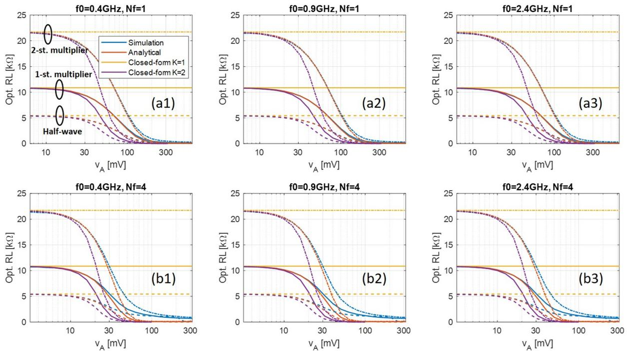
**Figure 3.** Optimal load calculated by transient simulation (blue), numerical solution of the analytical model (red), and closed-form solutions (yellow and purple), when (a)  $N_f = 1$ , and (b)  $N_f = 4$  with  $\Delta_f = 1$  MHz, with half-wave, 1-, and 2-stage voltage-multipliers using Skyworks SMS7630. The results under different frequency bands (a1,b1) 400 MHz, (a2,b2) 900 MHz, and (a3,b3) 2.4 GHz are shown, too.
