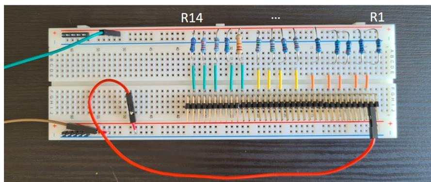
Figure 6. Resistor bank on a bread board.
