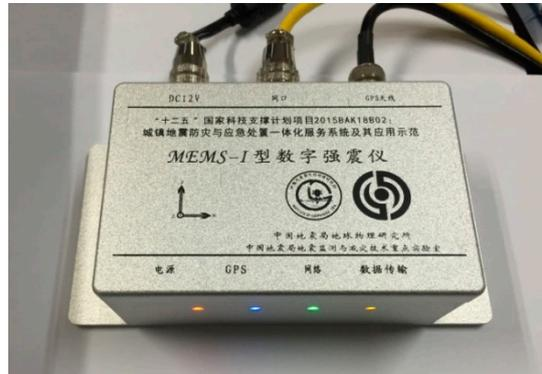
Figure 7. The MEMS seismic intensity rapid reporting instrument developed in this study.
