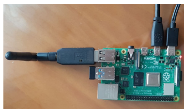
Figure 22. Raspberry pi 4 and zzh! providing gateway functionalities to integrate home sensors.
