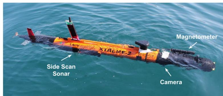
**Figure 14.** LAUV-Xtreme-2 AUV integrated with Side-scan Sonar, Underwater Camera and Magnetometer [140].
