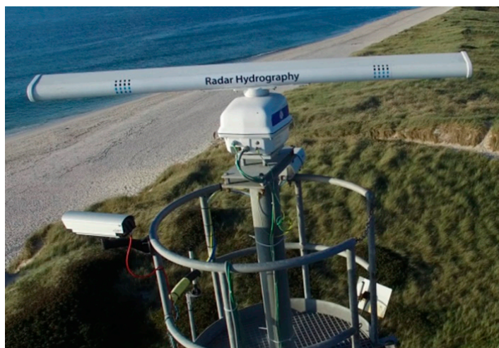
Figure 1. Coastal setup of the coherent on receive marine radar (MR) system on the Island of Sylt in the German Bight of the southern North Sea.
