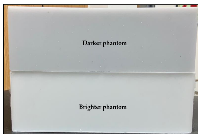
Figure 16. Darker and brighter silicone rubber phantoms.
