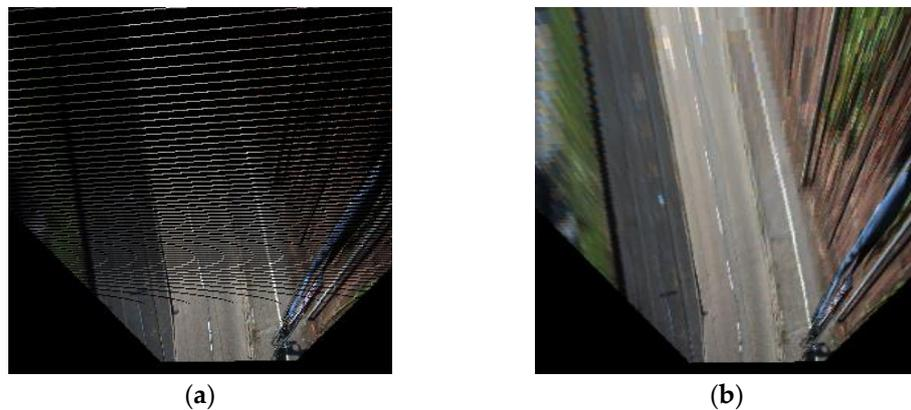
**Figure 3.** Different transformation methods. (a) Data transformed from image coordinates to bird's eye view coordinates and (b) data transformed from bird's eye view coordinates to image coordinates.
