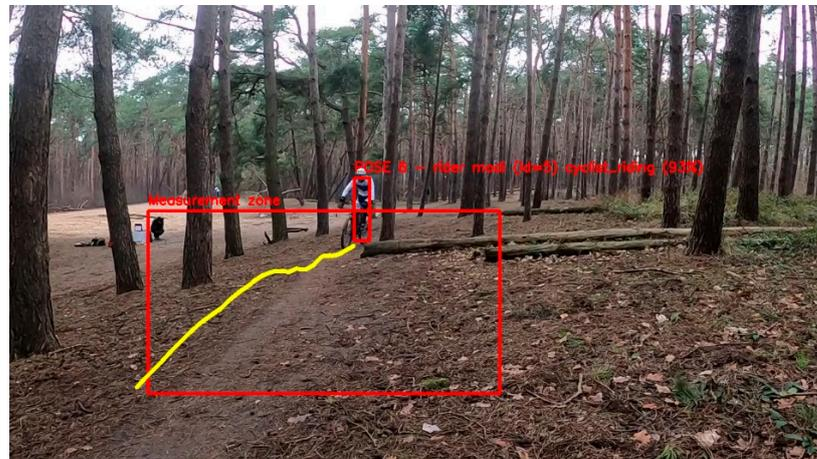
**Figure 2.** Illustration of the fence principle on a video frame of a cyclocross training session. The red rectangle is the region of interest. Results of pose detection, tracking, and post processing are illustrated by the yellow path within the fence.
