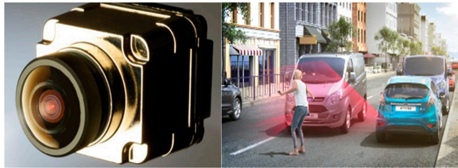
**Figure 7.** Pedestrian detection using SVC cameras. A Valeo 360 surround view camera could offer a three-dimensional view of the environment. (Image source: [www.valeo.com/en/360-vue/](http://www.valeo.com/en/360-vue/) and [www.fordclubsweden.se](http://www.fordclubsweden.se); accessed on 12 March 2021).
