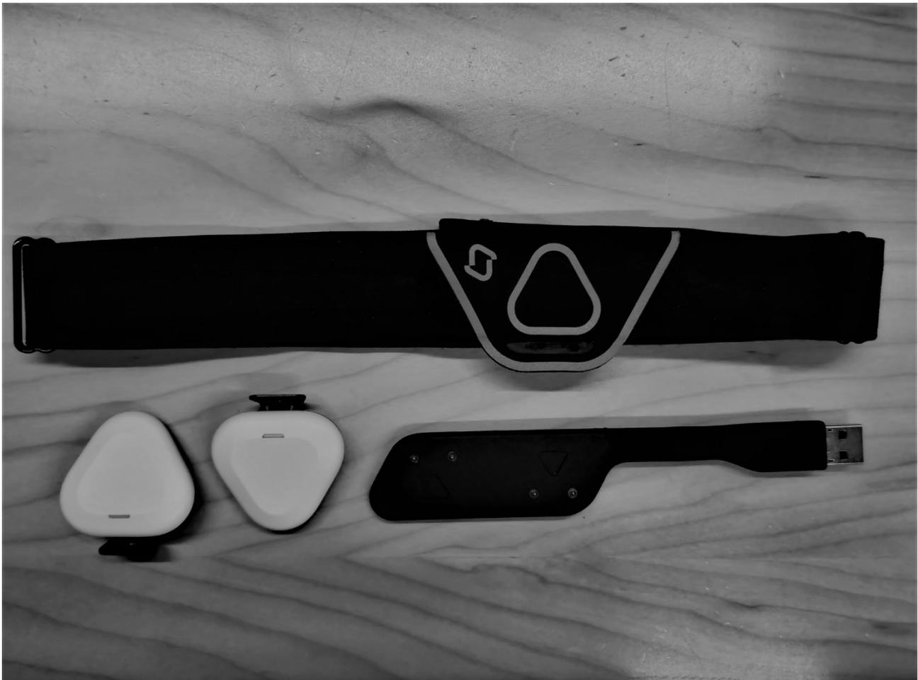
**Figure 1.** Components of the SHFT Device: A chest band, two pods, and a USB charger.
