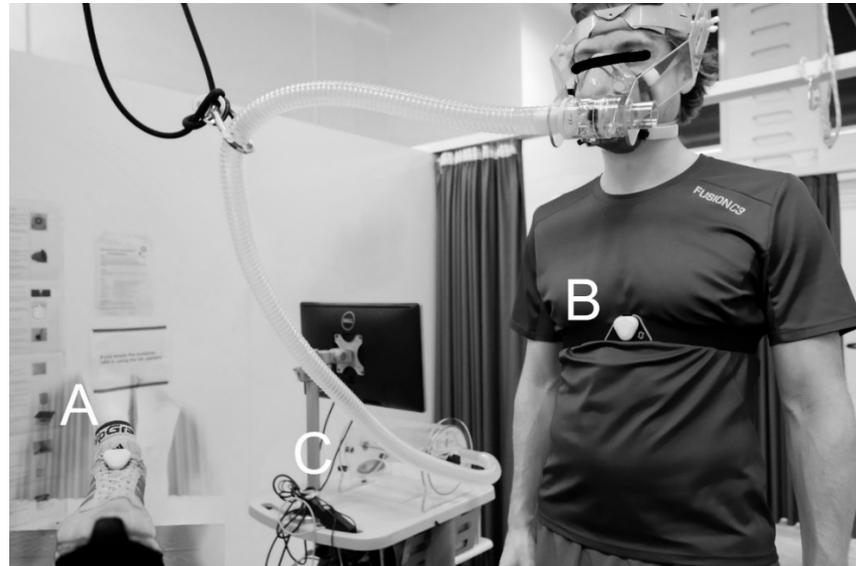
**Figure 3.** Demonstration of the indoor treadmill test setup where (A) illustrates a SHFT pod equipped on a random lace, (B) illustrates a SHFT pod equipped on a chest band, and (C) illustrates the mixing chamber positioned on a metabolic cart.
